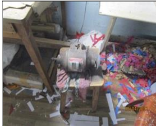
Photo of non-conformity wheel guard was not provided to grinding machine.JPG
